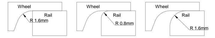
These examples use a flange root radius of 1.6mm and the gauge face of the rectangular rail is at the outer edge of the root radius. The first example has no railhead radius. The second has a railhead radius of 0.8mm. The third has a railhead radius of 1.6mm which is the same as the flange root radius.
